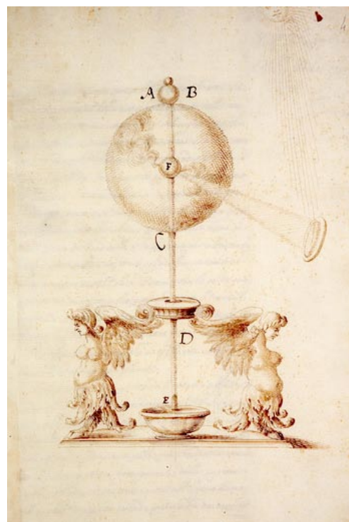
Drawing of the experiment on the behaviour of smoke in a vacuum, one of the experiments on the vacuum undertaken by the Academy of the Cimento (Biblioteca Nazionale, Florence, Ms. Gal. 289, c. 4r)
